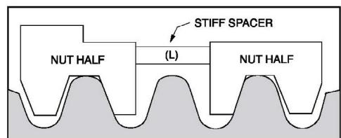
This gap ( $L + L_{I2}$ ) is now the amount of backlash which has developed in the unit. This backlash can be removed by replacing the stiff spacer with a new spacer equal to  $(L + L_{I1} + L_{I2})$ . This process, although effective, would be extremely costly and difficult to implement on a continuous basis.
