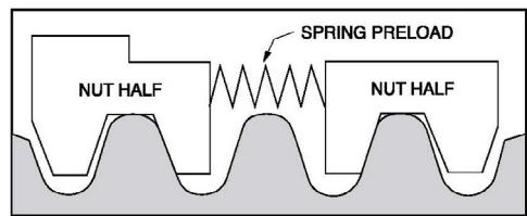
For example, if the maximum axial load to which the system is subjected is 50 lbs., the amount of spring preload must be equal to, or greater than, 50 lbs. in order to maintain intimate screw/nut contact. The problems arising from preloading in this manner are increased drag torque and nut wear. Obviously, the higher the load at the screw/nut interface, the higher the required torque to drive the nut on the screw and the more susceptible the unit is to nut wear.
