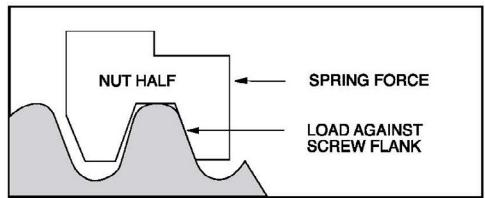
An alternate method replaces the spring with a stiff spacer sized to fit exactly between the two nut halves. There is no excessive preload force at the interface and the unit is capable of carrying high axial loads in either direction with no backlash. This is fine initially. However, as use time increases, wear begins on the nut threads causing a gap to develop between the spacer (L) and the nut halves.
