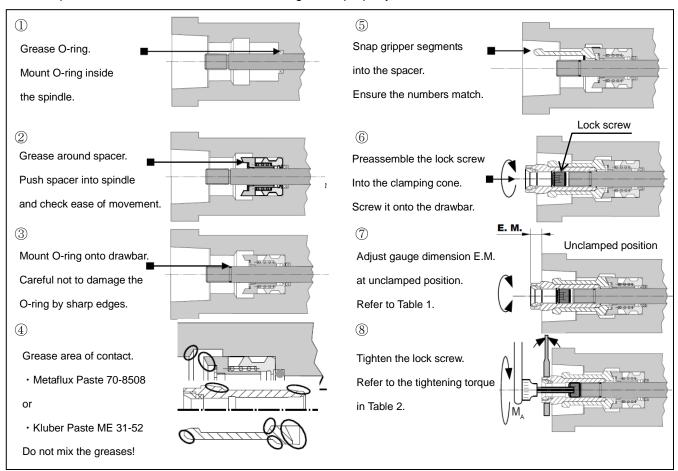
% Check E.M.dimension after approx. 100 tool changes. Retighten the lock screw through clamped tool.
