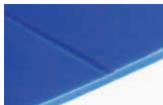
Butt welding with paddle welding tool
