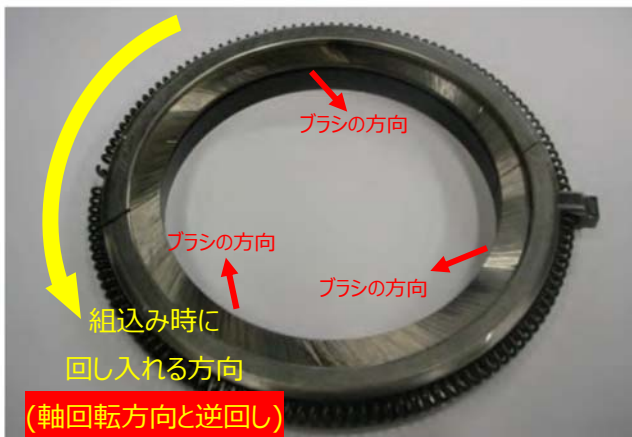
High Pressure Seal Side (Brush) 羽根車側 (ブラシ面)
